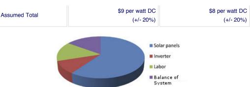
About 60% of the cost to install a solar-electric (PV) system goes to the solar photovoltaic (PV) panels, 10% to an inverter, 15% to direct labor, and 15% to the "balance of system" (BOS) costs.
